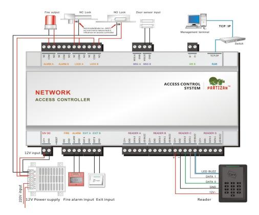
\*Note: the colour marking of the wires may vary from the one used in the scheme. Please check the code marking compliance for the correct connection of the device.
