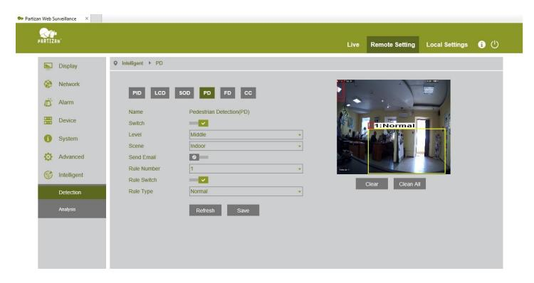
PD is used to detect the pedestrians in the traffic zones. Can be integrated to the "Safe City" systems. When detecting a pedestrian, the system will send an alarm notification and the object will be shown with graphic image.
