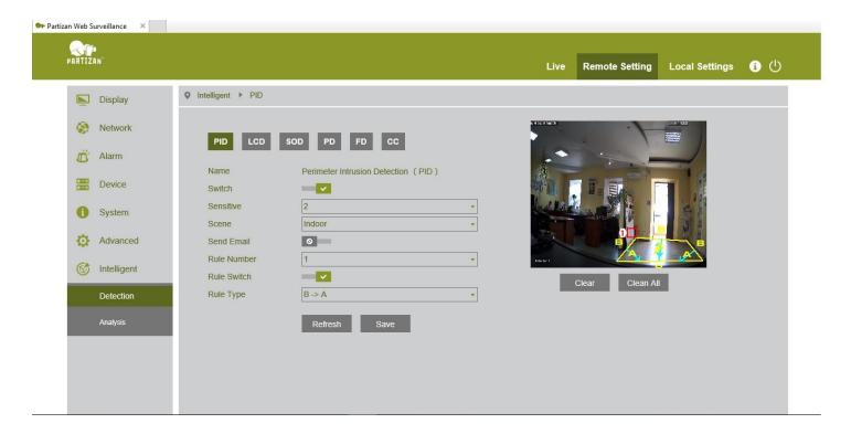
PID is used to secure the perimeter or open space. When the object is entering the zone which was previously marked, the system is making the alarm notifications. The object and its trajectory will be shown with the graphic image.
