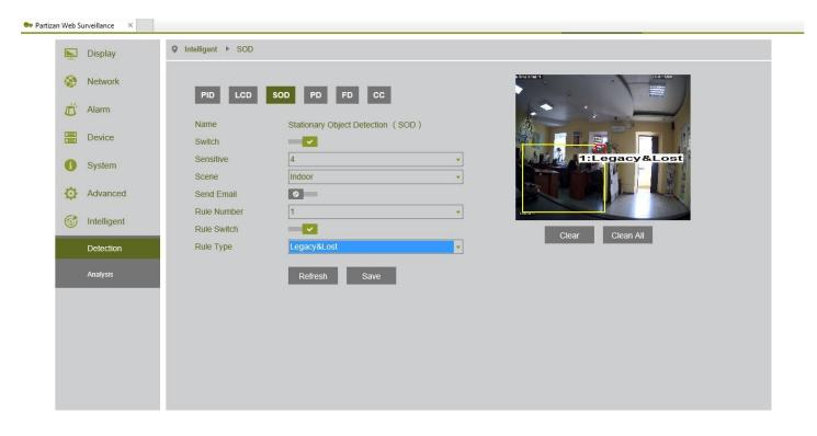
SOD is used for detecting if the static object appeared in or was removed from the marked zone. For example, for public places to prevent robbery or to detect the potentially dangerous objects. When detecting the system will send the alarm notifications and the object will be shown with the graphic image.
