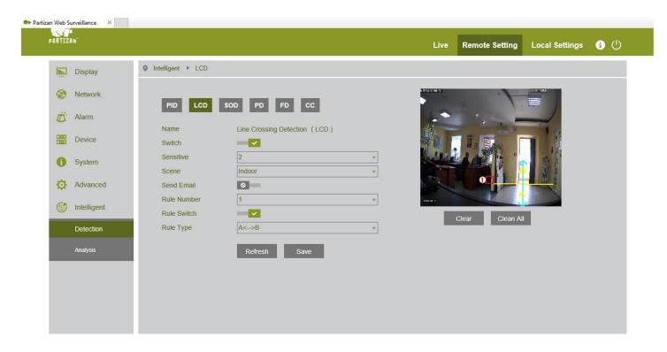
LCD is used to secure open spaces or spaces with limited access. When crossing the virtual line, the system is making the alarm notifications. The object and its trajectory will be shown with the graphic image.
