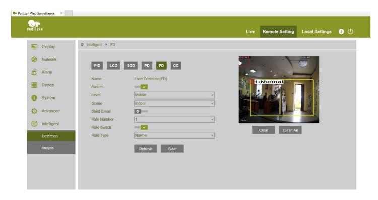
FD is used to detect faces in the frame (not the Face Recognition) and for further basic search in the archive. When detecting, the system will send an alarm notification and the face will be shown with graphic image.
