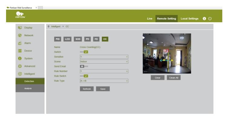
CC is used to calculate how many times the line has been crossed by the objects, For example, the rough calculation of the visitors in the mall or shop. When detecting, the system will send an alarm notification and the object will be shown with the graphic image. Number of crossings for enter (IN), exit (OUT), total amount (Total) will be shown by the counter in the left top corner of the frame.
