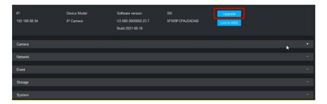
In the window that opens, select the folder with the previously saved firmware. Select the file and click the **Firmware** button.
