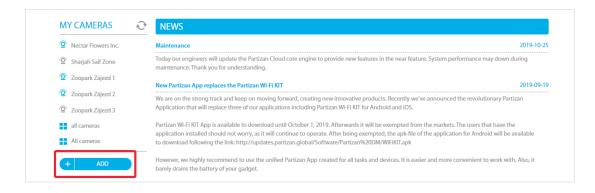
3. To enable PUSH messages, you have to activate the option "Arm the camera". In the left part of the window, in "MY CAMERAS" menu, hover over the desired camera and click on the settings icon to the right of the device name
