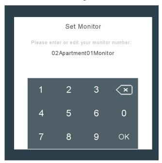
**Apartment** - button number on the calling panel (from 01 to 04) **Monitor** - intercom number (01 - main intercom) Ready? Press "OK"!
