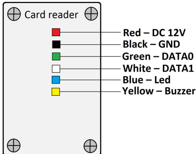
\*Note: the colour marking of the wires may vary from the one used in the scheme. Please check the code marking compliance for the correct connection of the device.
