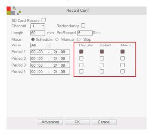
7. In the Manual and Stop modes it is impossible to set the time period and mode of recording
