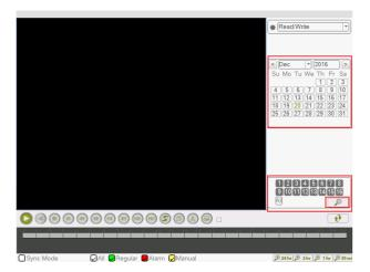
4. In the band that appears on the screen select the time and press the **Play** button on the toolbar.
