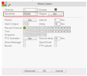
6. Select the camera or a group of cameras from which the recording will be made in case of motion detection on the channel selected in item 3.
