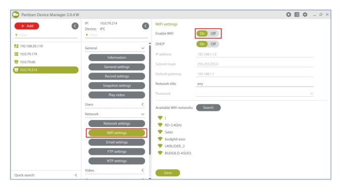
2. Configure the network settings manually or enable DHCP option.
