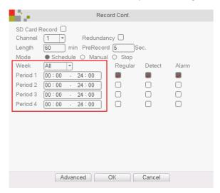
6. Choose the recording start mode – based on motion detection, continuous recording or on alarm.
